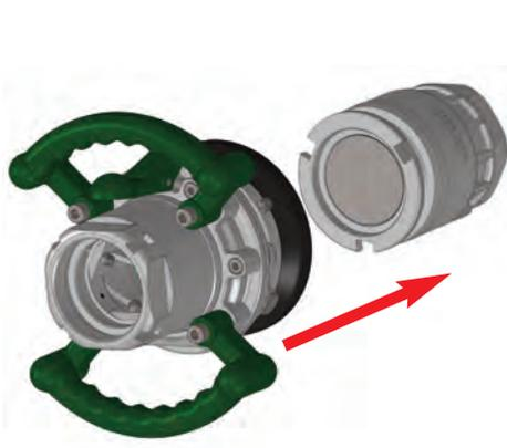
1. The coupler (hose unit) is pushed over the adaptor (tank unit) without canting until the three rollers - offset by 120° - of the coupler have been completely guided through the slots of the adaptor. The position is not relevant.
