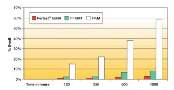
In a standard immersion test **Perlast® G80A** shows little volume swell even after 1000 hours @ 250°C.
