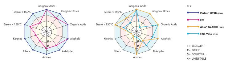
The performance of ETP terpolymer is close to a perfluoroelastomer, however its maximum temperature is 210°C (410°F).
