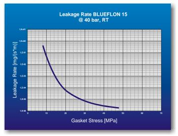
Even at low gasket stress **Blueflon** shows very good sealing properties.
