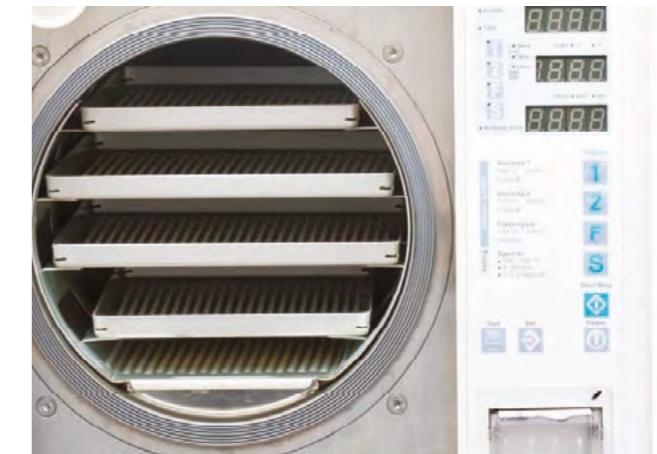
Moist heat technology is the most widely used method of sterilization. RUBBERFLATE® inflatable seals made out of heat and water resistant materials can provide safe sealing solutions for applications in this area.
